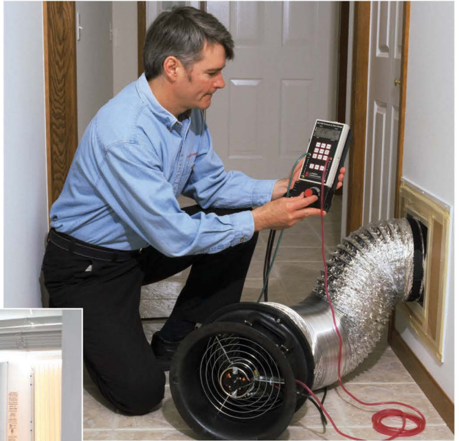
A duct-blast test can identify air leaks in your home's ductwork.
